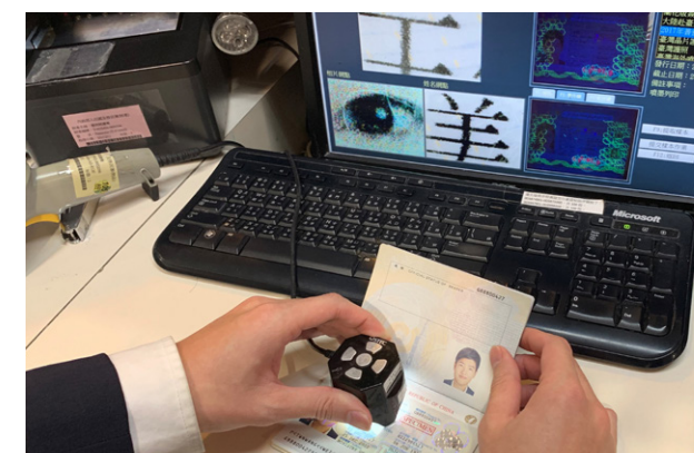
The Suspicious Passport Comparison System is used to compare a problematic passport
